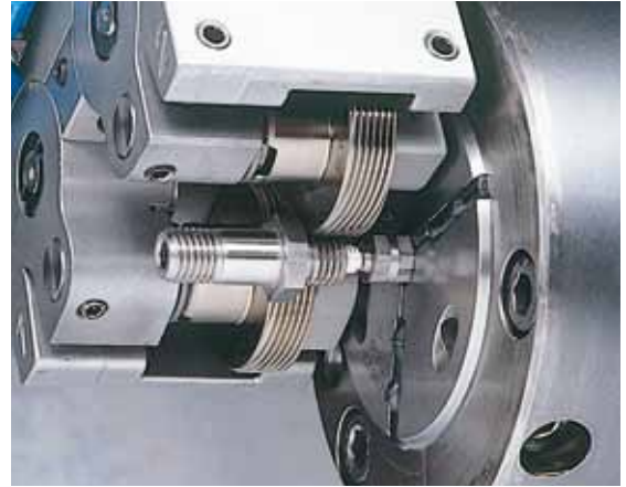
Thread rolling behind a collar
